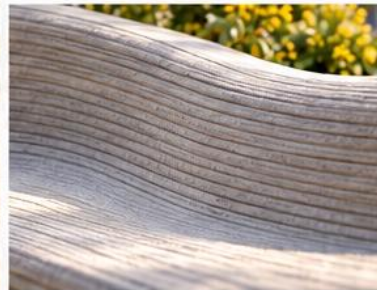
03 LAYERED CONCRETE Visible horizontal print courses.
